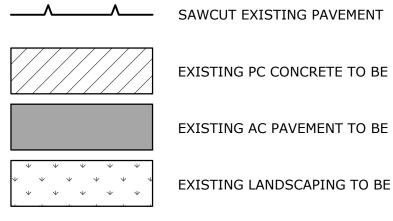
EXISTING PC CONCRETE TO BE REMOVED EXISTING AC PAVEMENT TO BE REMOVED EXISTING LANDSCAPING TO BE REMOVED
