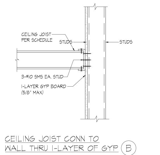
TYPICAL CEILING JOIST AND CONNECTIONS TO WALLS
