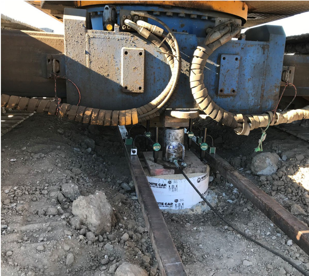
Figure 1. AGI Load Test 1 Setup
