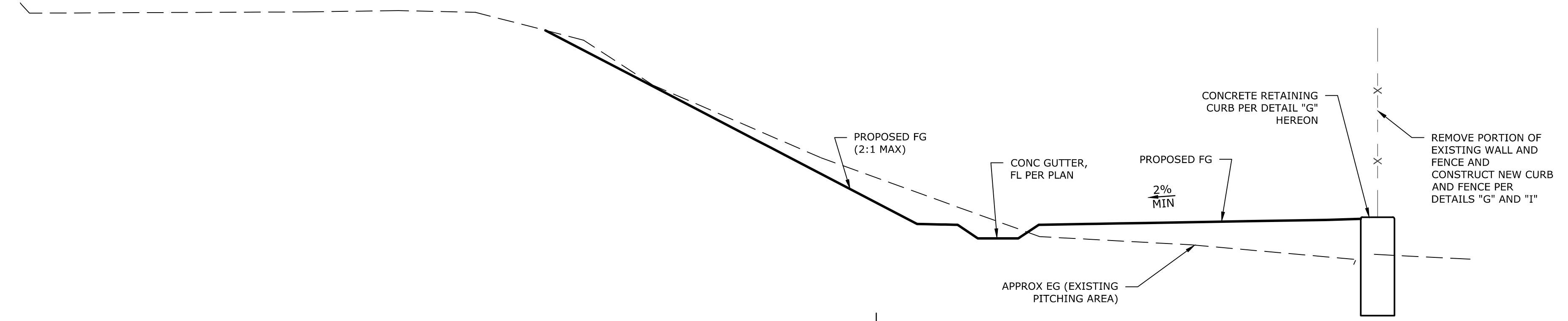
SECTION NEAR PITCHING AREA B 1"=2'
