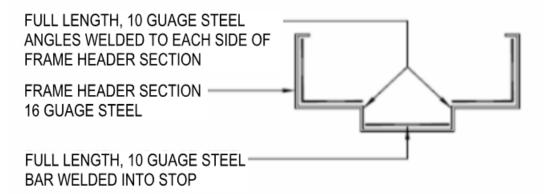
MOORPARK COLLEGE HSC – BIO-MFR PROGRAM VENTURA COUNTY COMMUNITY COLLEGE DISTRICT DETAIL # 3 - CONCRETE WALL CONDITION DETAIL FOR EXTERIOR DOOR WHERE RAIN DRIP IS REQUIRED. EXTERIOR SIDE WITH 22 GAGE GLAVANIZED SHEET METAL OR PAINT LOCK RAIN DRIP WELDED IN PLACE.
