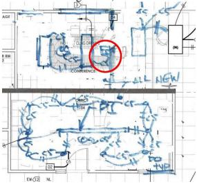
a. A – The wall switch in the old conference room is a switch which is a D2 type in the RED circled area.
