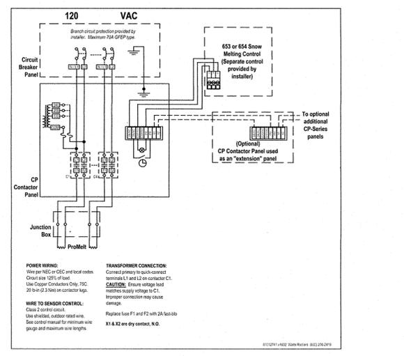
**POWER WIRING:** Wire per NEC or CEC and local codes. Circuit size 125% of load. Use Copper Conductors Only. 30' or (2.3m) on conductor legs. Breaker connection may cause damage.
