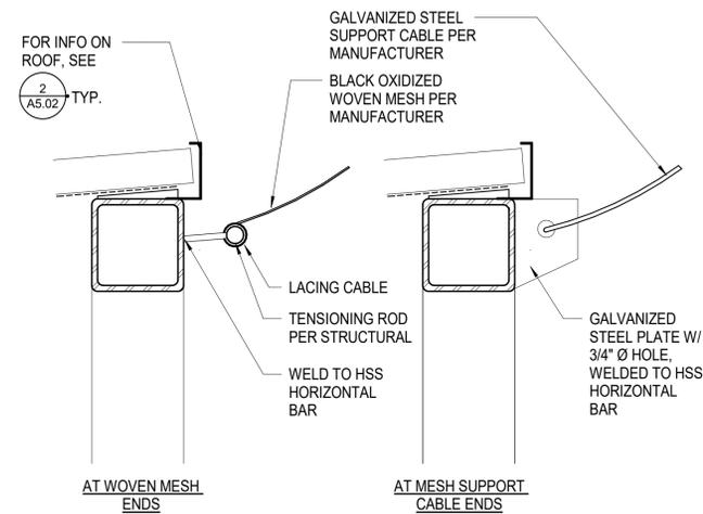
**7** WOVEN MESH TO HSS TUBE DETAIL
