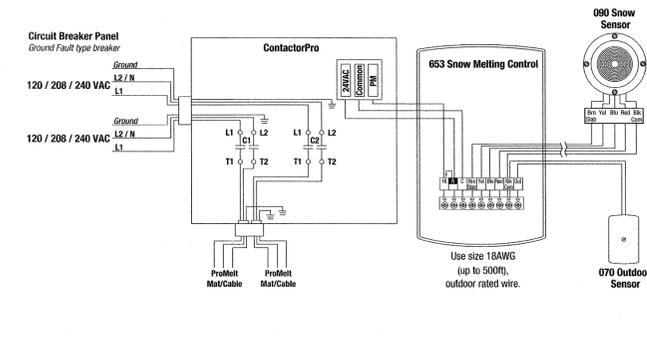
ProMelt Snow Melting Control Kit PM-L2 with ProMelt Mat(s) or Cable(s)
