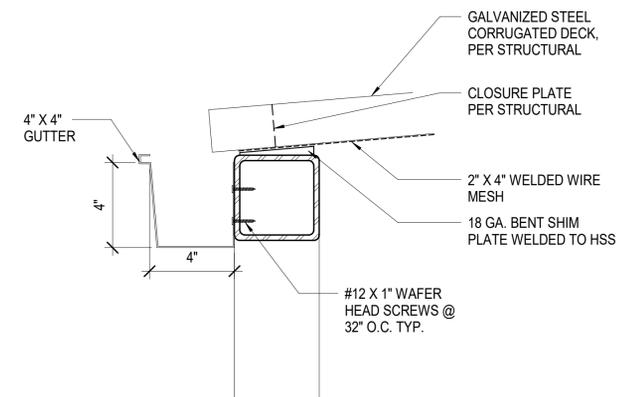
**4** ROOF AND GUTTER DETAIL
